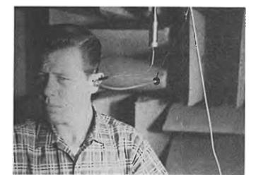
FIG. 2. Photograph showing the subject, the earmold with driver, and the pressure measurement probe connected to condenser microphone on its preamplifier. Note that the driver system and the pressure measurement system are mounted from the anechoic wedges so as to be mechanically isolated from the subject. Subject's chair is mechanically isolated from the floor.
