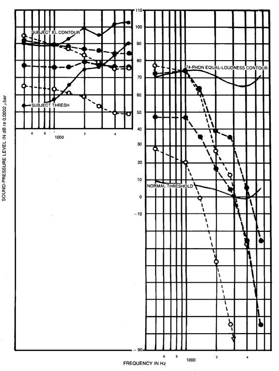
FIG. 6. Solid dots and heavy dashes show the effect of the hearing-aid compression of Fig. 4, without equalization. Open circles outline speech bands before compensation.
