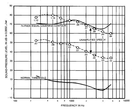
FIG. 1. Sound-pressure levels of conversational speech, as measured in  $\frac{1}{2}$ -oct bands by Dunn and White (1940). Numbers under open circles show the proportionate positions of speech levels relative to the amplitude range between normal threshold and the ISO 74-phon equal-loudness contour.
