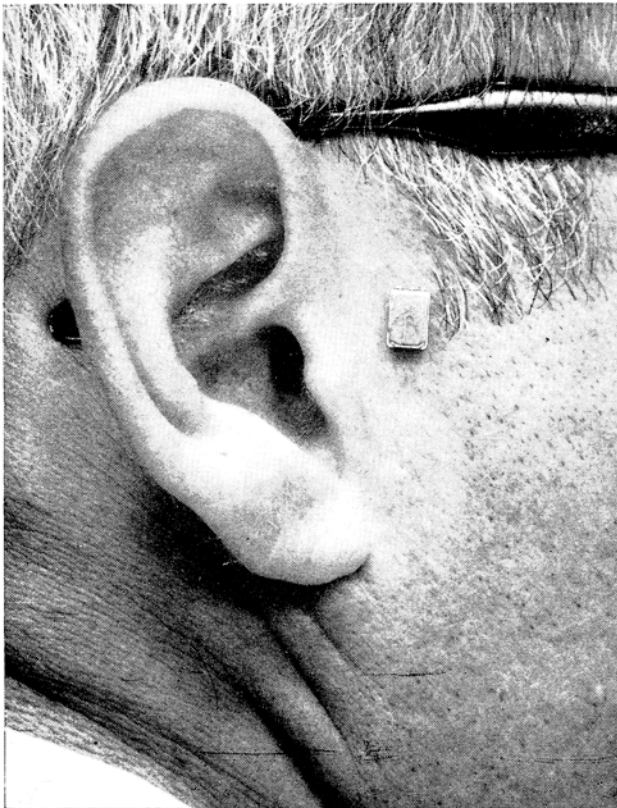
Fig. 7. Ceramic microphone shown next to a human ear.
