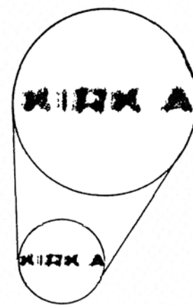
Fig. 5. Visual illustration of a clarity problem that is not helped by additional magnification. Fuzzy images (or sounds) remain fuzzy upon magnification (or amplification).
