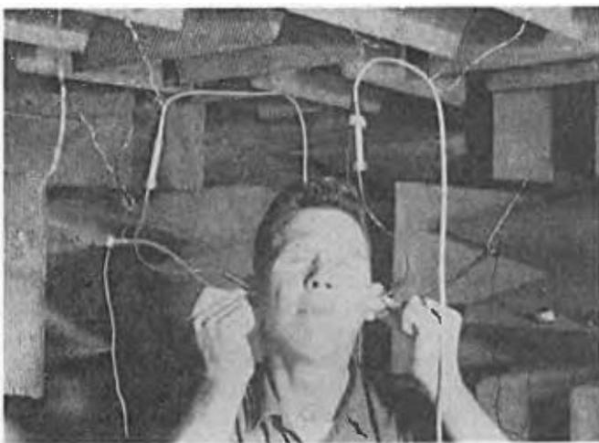
FIG. 8. Photograph showing the experiment arrangement of the probes and the cone type driver systems. When the subject removed the cones to listen to the loudspeaker source, the cones were held near the ear canal and the probe system measured the pressure level of the free-field stimulus.
