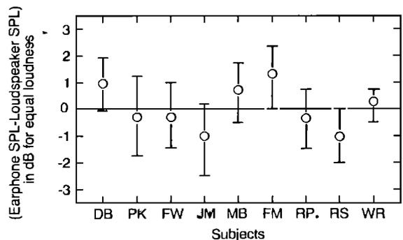
FIG. 14. The results of binaural loudness balancing at 100 Hz for various subjects using earphones in cushions as one source and a loudspeaker (with earphones off the ears) as the other source. Average differences for each subject in sound pressure levels are plotted. The subject's chair was mechanically isolated; the SPL range was 65–85 dB; and the bars are 95% confidence intervals.
