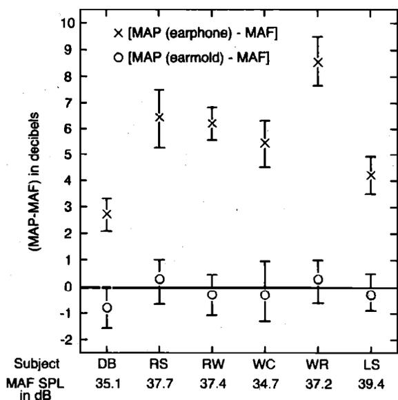
FIG. 3. Threshold differences between pressure thresholds (MAP: earphone or earmold source) and free-field thresholds (MAF: loudspeaker source). Monaural listening with opposite ear properly occluded. Frequency 100 Hz; bars are 95% confidence intervals.
