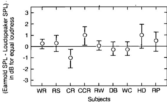
FIG. 12. The results of monaural loudness balancing at 100 Hz for various subjects using the conical earmold-driver system as one source and the loudspeaker as the other source. The nonlistening ear was properly occluded; the subject's chair was mechanically isolated; the SPL range was 65–85 dB; and the bars are 95% confidence intervals. ( $N$  typically ranged from 20 to 30 over four or five different days.)
