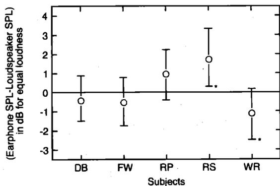
FIG. 15. The results of binaural loudness balancing at 100 Hz for various subjects using earphones in cushions as one source and a loudspeaker (with earphones left on the ears—no signal voltage on earphones) as the other source. Average differences for each subject in sound pressure levels are plotted. The subject's chair was mechanically isolated; the SPL range was 65–85 dB; and the bars are 95% confidence intervals. (\*N for these data ranged from 6 to 10.)
