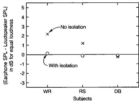
FIG. 10. Chair vibration effects. The differences in sound pressure level from an earphone source and from a distant loudspeaker source are shown for three subjects performing binaural loudness balances for 100-Hz signals from the two sources. One set of data was obtained with the subject's chair in direct contact with the woven wire floor of the anechoic chamber (no isolation). The other set was obtained with the subject's chair mechanically isolated from the chamber floor.
