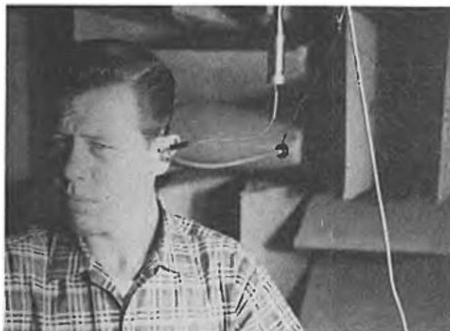
FIG. 2. Photograph showing the subject, the earmold with driver, and the pressure measurement probe connected to condenser microphone on its preamplifier. Note that the driver system and the pressure measurement system are mounted from the anechoic wedges so as to be mechanically isolated from the subject. Subject's chair is mechanically isolated from the floor.
