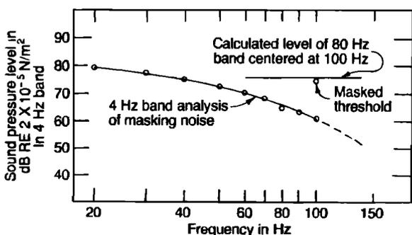
FIG. 6. Simulated physiological noise used in masking experiments to verify the critical bandwidth for monaural masking of 100 Hz due to this type of spectrum. With the noise adjusted as shown, subjects adjusted the level of a 100-Hz tone to obtain their masked thresholds. The average value of their masked thresholds was within 1 dB of the calculated level of the energy in an 80-Hz band centered at 100 Hz due to the masking noise.
