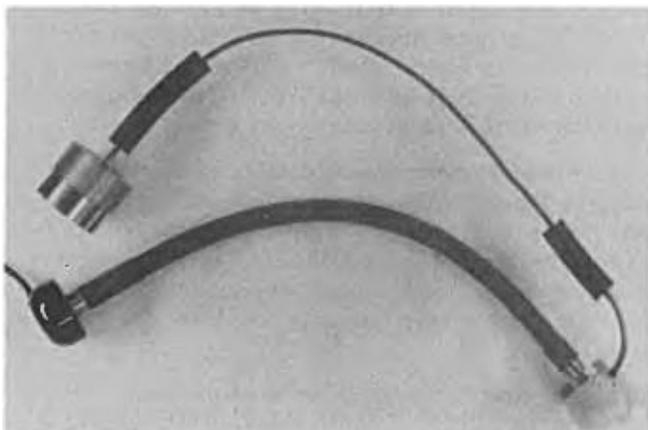
FIG. 1. Photograph showing earmold coupled to hearing aid driver unit via rubber tubing. Enclosed volume is 6 cm<sup>3</sup>. Pressure in the ear canal is measured by the probe tube connected to a standard 2.5-cm condenser microphone.
