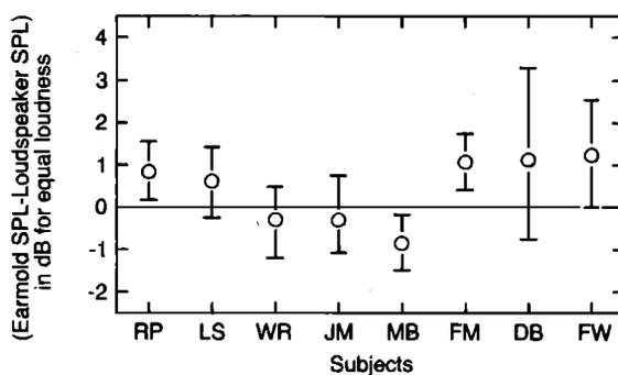
FIG. 16. The results of binaural loudness balancing at 100 Hz for various subjects using the conical earmold pressure system as one source and a loudspeaker (conical earmolds out of the ear canal) as the other source. Average differences for each subject in sound pressure levels are plotted. The subject's chair was mechanically isolated; the SPL range was 65–85 dB; and the bars are 95% confidence intervals.
