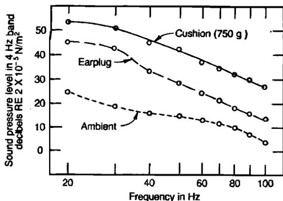
FIG. 5. Average physiological noise in 4-Hz band at the entrance of the ear canal when the ear was covered by a cushion and a conventional earphone (no electrical signal on earphone) with a force of 750 g holding the cushion against the pinna (top curve); when the earmold system was in the ear (middle curve); and the ambient noise spectrum measured at the ear with the ear canal open (lower curve).
