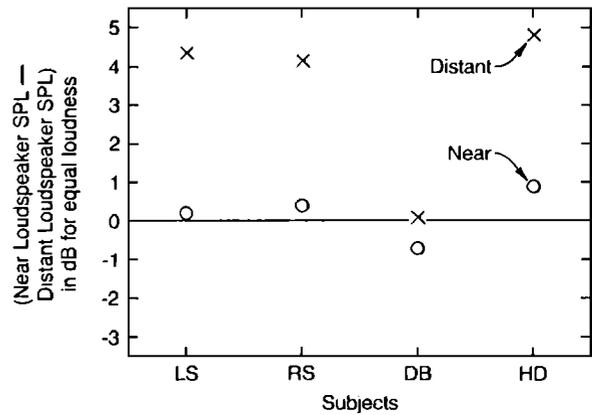
FIG. 9. The source location effect. The results shown are for four subjects performing monaural loudness balances between a loudspeaker near the head and a loudspeaker located across the anechoic chamber (about 4–5 m) from the subject. Differences in sound pressure level between the near source and the distant source are shown for a frequency of 100 Hz. Subject's chair was mechanically isolated from the floor. The subject's nonlistening ear was occluded with an earplug covered by earmuff.
