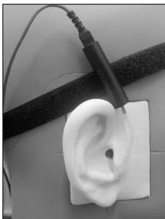
Fig.1b Probe placement in ear with headband (option 2)
