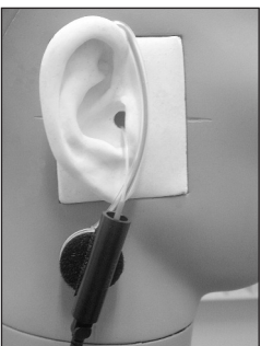
Fig.2 Probe placement in ear with earhook.
