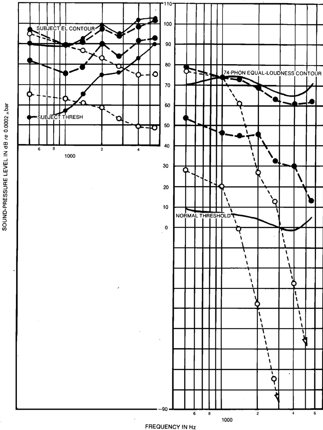
FIG. 4. Solid dots and heavy dashes show the effect of the compromise hearing-aid compensation (two-channel compression plus post-compression frequency equalization) described in Sec. V. Open circles at the right outline processed speech before compensation, as in Fig. 2, and open circles at the left outline amplified, unprocessed speech before compensation.
