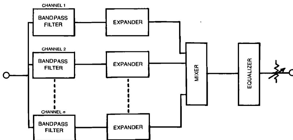
FIG. 3. Signal processor to simulate for normal listeners the abnormal loudness relationships perceived by a deaf subject with recruitment. The processor is an electrical analog of recruitment: The response of the model represents the deaf subject's loudness response relative to normal response.
