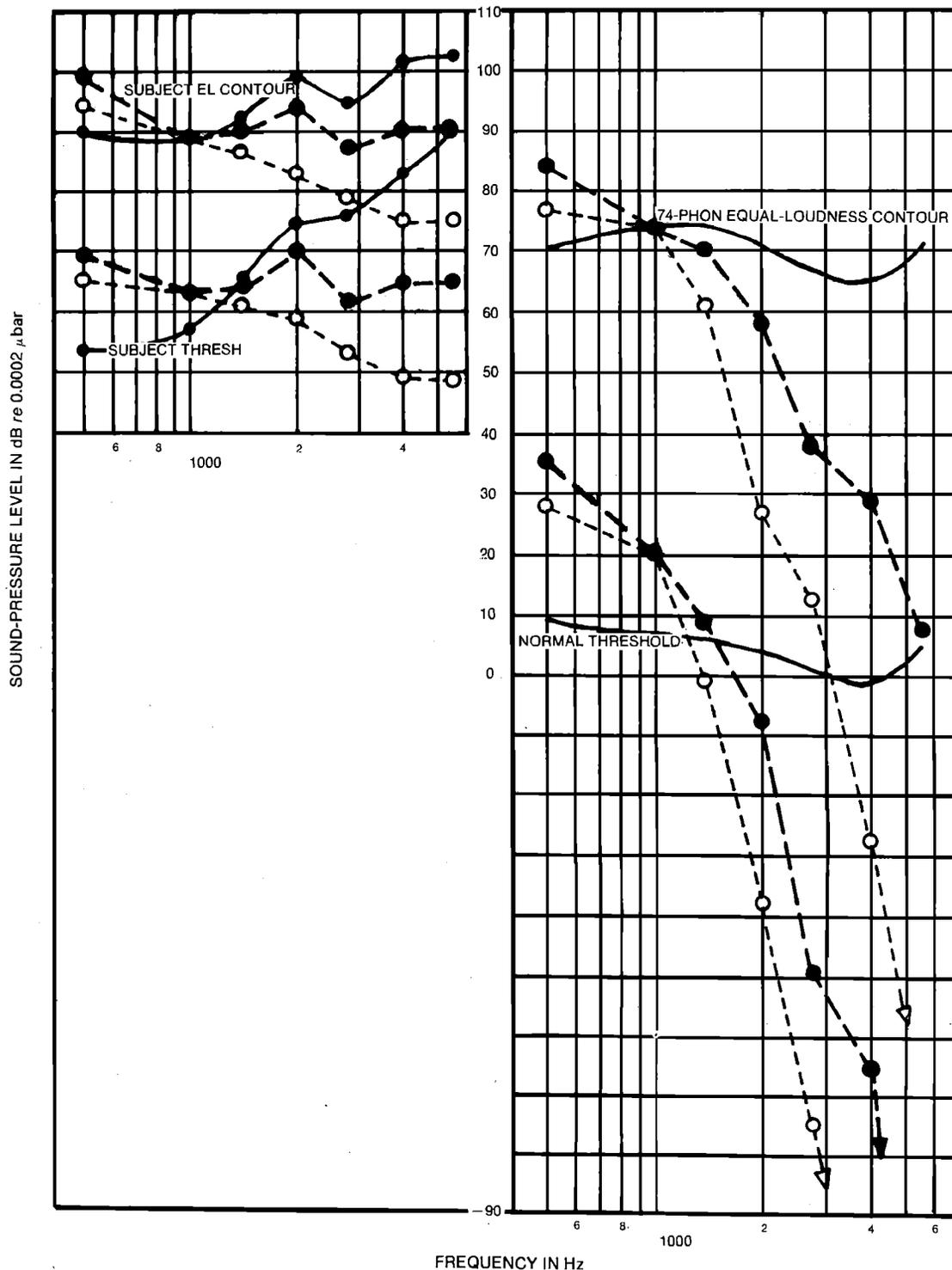
FIG. 5. Solid dots and heavy dashes show the effect of the hearing-aid equalization of Fig. 4, without compression. Open circles outline speech bands before compensation.
